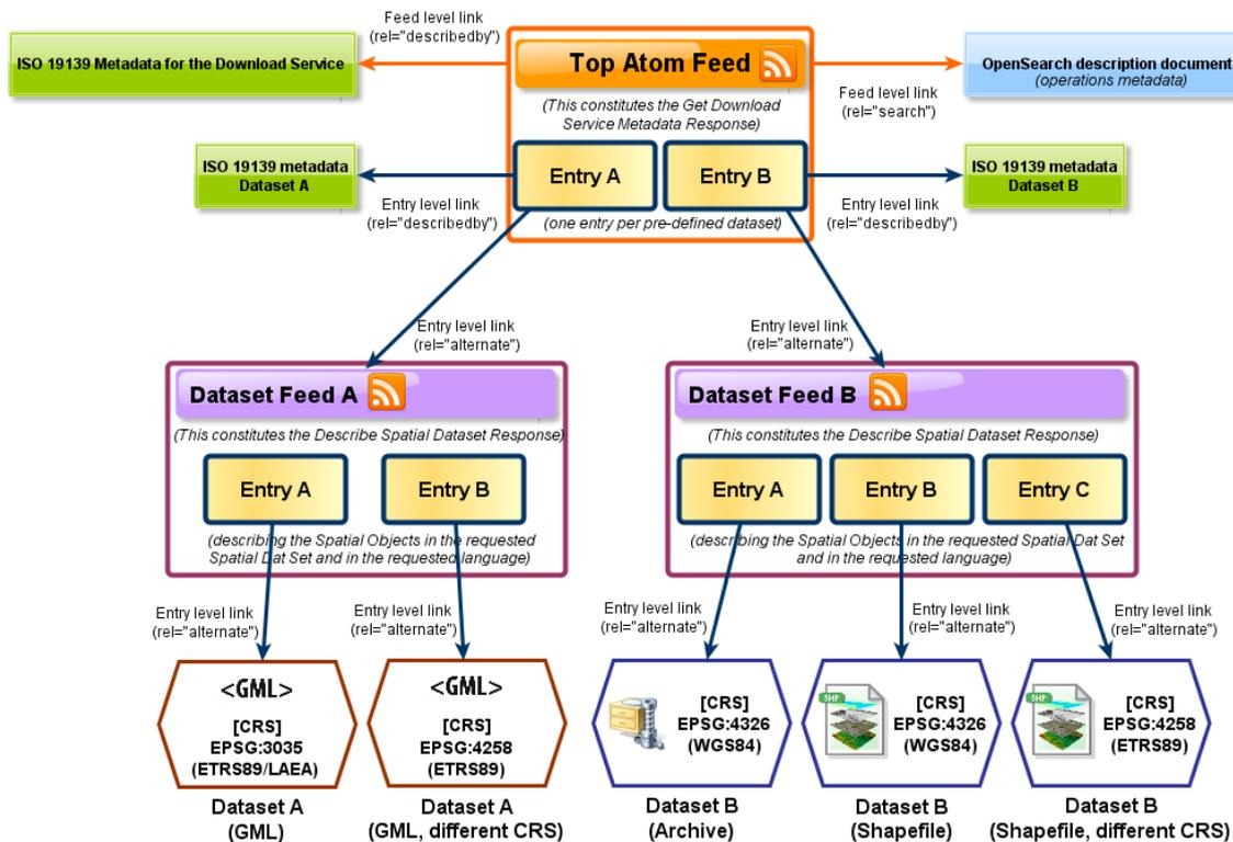
Figure 5 Overview of Atom feed structures
