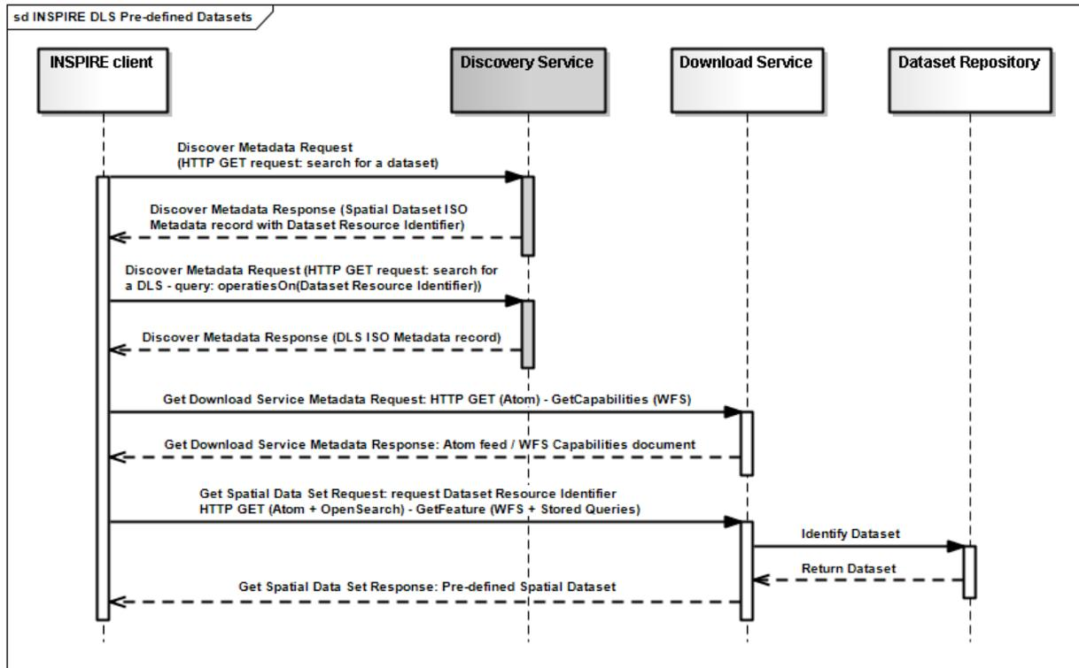
Figure 2: Simple sequence diagram showing download of datasets via a pre-defined download service
